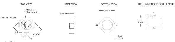
Dimensions are in millimeters
